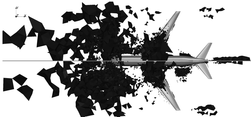
Fig. 3 Case 1.1 medium grid: field elements of local dissipation error of pitch moment coefficient larger than 1.5 \cdot 10^{-7} (bottom) and drag coefficient larger than 7 \cdot 10^{-9} (top). Top view.
